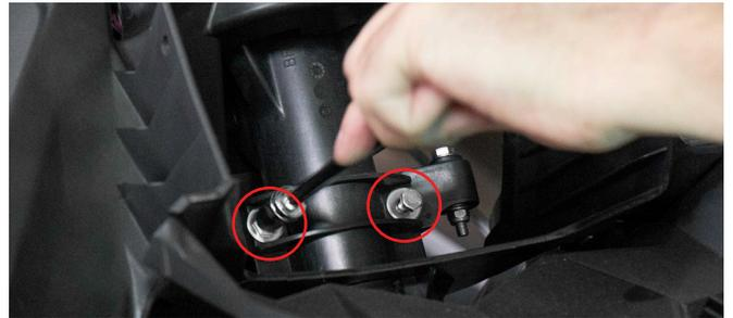
6. Undo the 10mm nyloc nut and bolt, connecting the steering arm to the clamp.
