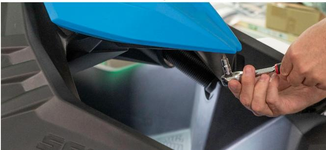
5. Undo the steering clamp by removing the 2 x 10mm bolts.
