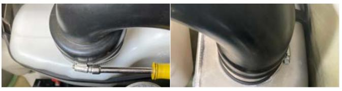
**3.** Remove sound suppression baffle straps and elbow hose connected to thru-hull fitting. Discard baffle. Retain OEM clamp.
