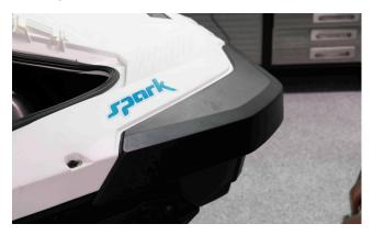
Australia: 10B 354 Brisbane Rd Arundel QLD 4214 Phone: +61 7 5563 1031 info@worx.com.au | worx.com.au United States: 9251 Orco Parkway Unit G, Riverside CA 92509 Phone: (951) 684-9679 info@worxracingusa.com | worxracingusa.com **16.** Undo the 16 torx bolts on the white plastic around the rear of the ski.
