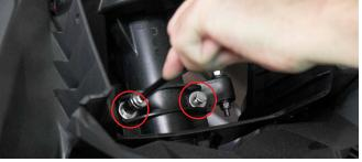
**6.** Undo the 10mm nyloc nut and bolt, connecting the steering arm to the clamp.
