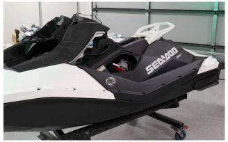
Remove the hull lifting up and toward the front of the ski so that the steering arm slides through the grommet.
