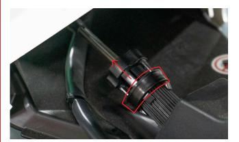
**9.** Undo the connection by spinning clockwise until it's removed.
