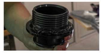
**23.** From the inside of the hull, plasce the outlet through the oem outlet position with the thread facing outside.
