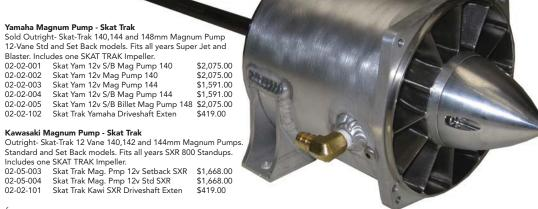
Designed with the freestyler in mind, the freestyle pump cone allows the engine to rev faster for the big tricks. Its small size lets a large volume of water move through the pump with less restriction than with the stock tailcone. This gives you more low end thrust for bigger air. Works great with a bored out stock nozzle to help provide even more low end. Detailed instructions and hardware included.
